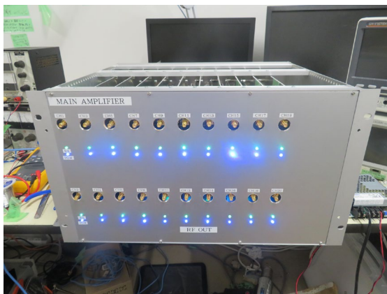
Figure 1. Photo of the main amplifier (left) head amplifier (right) for the 20-channel imaging receiver system, now under development and to be installed at the SuperDARN Hokkaido East radar site.
