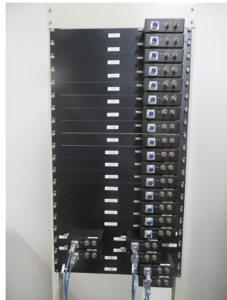
Figure 1. Photo of the main amplifier (left) head amplifier (right) for the 20-channel imaging receiver system, now under development and to be installed at the SuperDARN Hokkaido East radar site.
