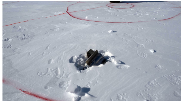
Figure 2. The dummy penetrator dropped from 75 m height in Antarctica.
