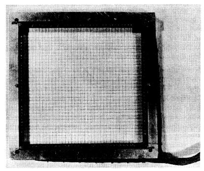
Fig. 5. Proto-type of two-dimensional current probe. 32 tungsten wires (0.15 mm in diameter) are stretched in horizontal and vertical directions, respectively. The spacings between the parallel wires are 5 mm. They are connected to multiplexers for the respective directions. The effective measurement area is  $15.5 \times 15.5$  cm<sup>2</sup>. The effective transparency of the two-dimentional probe is 94%.
