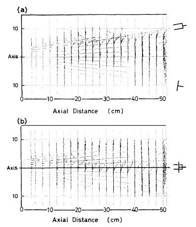
Fig. 8. (a) A series of radial distributions of the electron beam. They are projected onto the horizontal plane. (b) Those projected onto the vertical plane, which shows that the current trail deviates upward due to  $E \times B$  drift from the initial horizontal plane.
