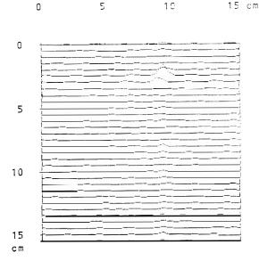
Fig. 6. An example of cross-sectional distribution of electron beam current measured by the two-dimensional current probe.
