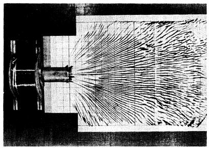
Fig. 1. Magnetic lines of force formed by a solenoid coil. They are emerged by iron powder. These field directions are consistent with direct measurements and calculated values. This field configuration is formed in the vacuum chamber for the present experiment. The maximum intensity of the magnetic field in the converging region is 350 Gauss.
