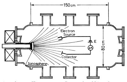
Fig. 2. Experimental setup. Electron source, collector and model ionosphere are arranged in a horizontal plane which includes the main axis of the magnetic field. The gas pressure in the chamber is order of 10<sup>-6</sup> Torr.
