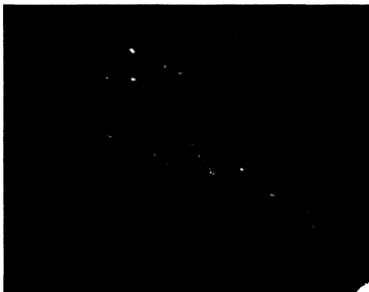
Fig. 1g. Cu-distribution picture. Cu does not show any uniform distribution, although a good part of it is dissolved in the Ni-rich phase. An overall enrichment of copper in the Ni-rich phase compared to troilite or kamacite is visible. In addition, copper occurs in the form of copper nodules at the phase boundaries between the kamacite inclusion and the Ni-rich phase surrounding it as well as at the upper left part at the Ni-rich metal/troilite boundary. A few additional nodules occur at the rhabdite/troilite interface.
