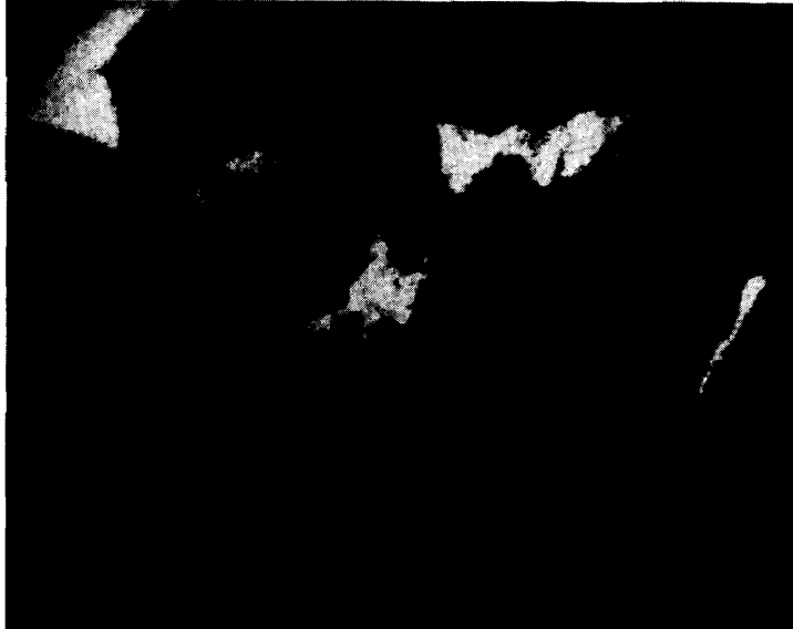
Fig. 3c. Sulphur distribution picture. It can be seen very clearly that there are troilite inclusions within the chromite inclusion (which is itself placed at the border of a large troilite nodule).
