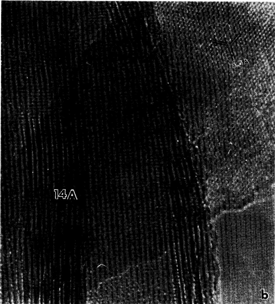
*Figs. 11a, b. High resolution electron micrographs of groundmass phyllosilicates (Y-791198). 14Å chlorite was observed for the first time in carbonaceous chondrite.*
