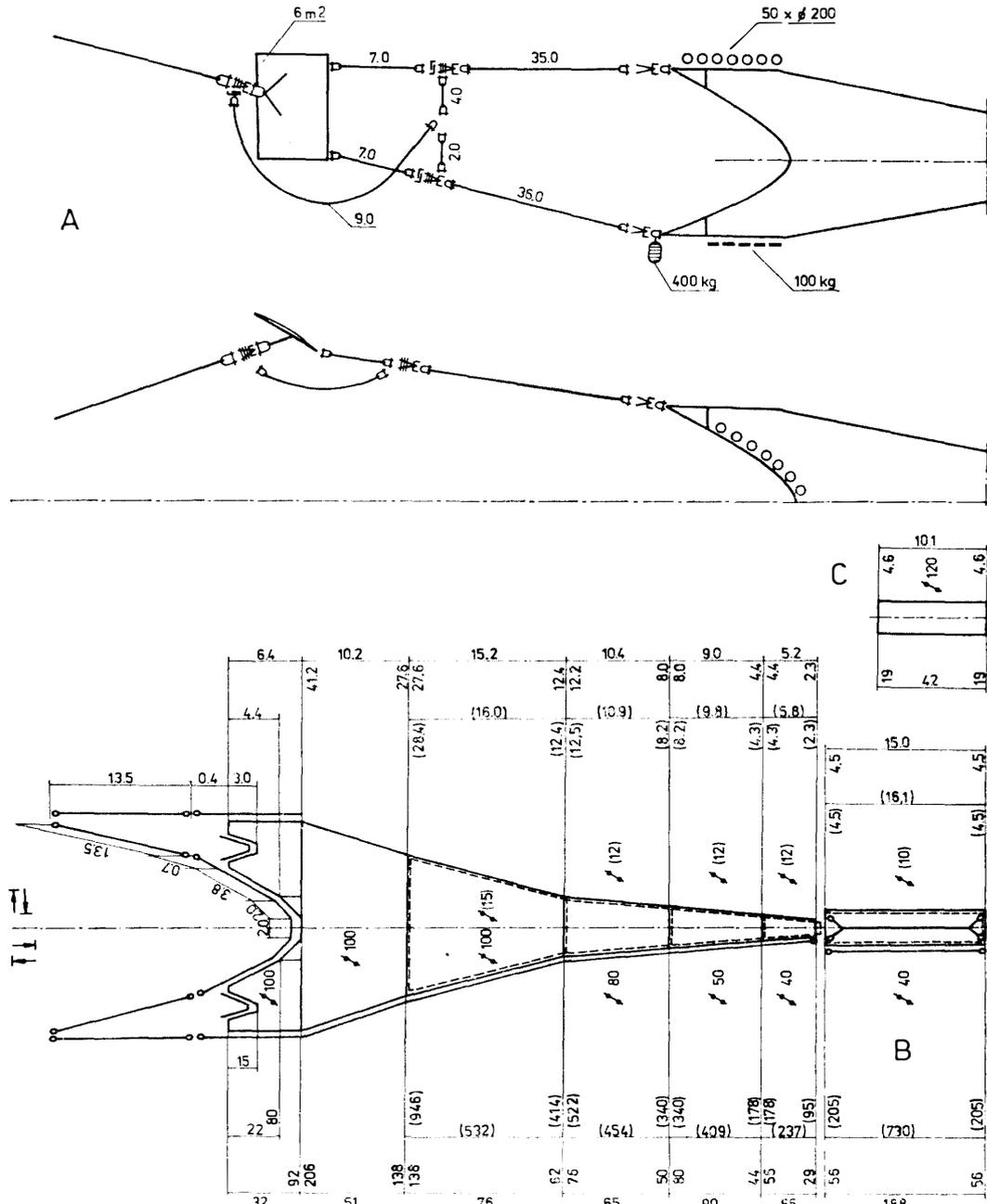
Fig. 1. General layout plan of the 368-mesh midwater sampling trawl (MST 16/41x4) designed by the Sea Fisheries Institute in Gdynia for sampling juvenile fish in SIBEX (redrawn from unpublished working plans after MODERHAK and KRĘPA). A: gear rigging, B: two-panel codend, C: outer covering of codend.
