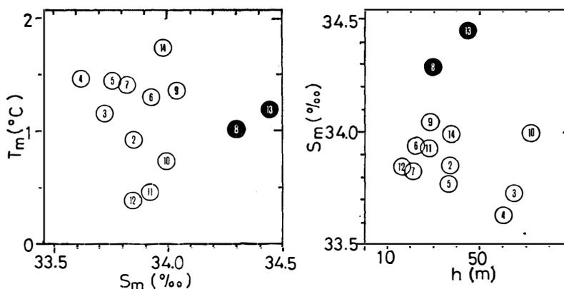
Fig. 10. Relations between  $T_m$  and  $S_m$  and between  $S_m$  and  $h$ . Symbols correspond to station symbols used in Figs. 4 and 7. No sea ice is estimated to form at Stns. 8 and 13. Sea ice is estimated to form at other stations.
