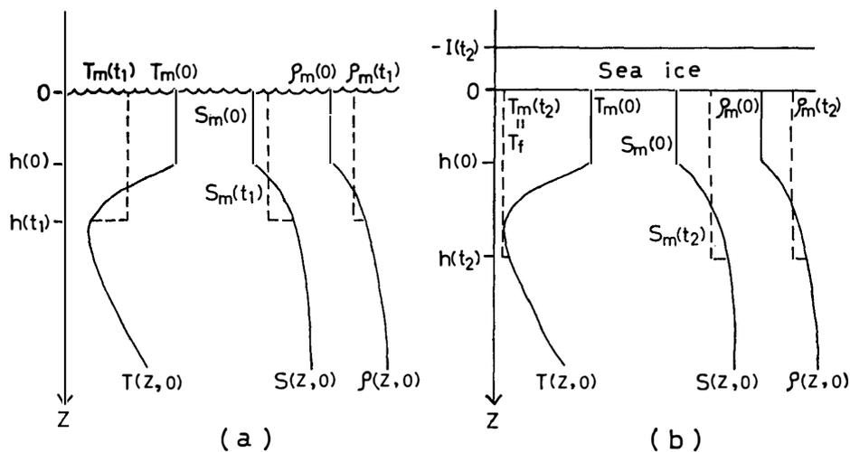
Fig. 1. Observed profiles (solid lines) of temperature  $T(z,0)$ , salinity  $S(z,0)$  and density  $\rho(z,0)$ , which are used as the initial conditions in the present model. Vertical broken lines indicate the calculated profiles (a) before freezing and (b) after freezing.
