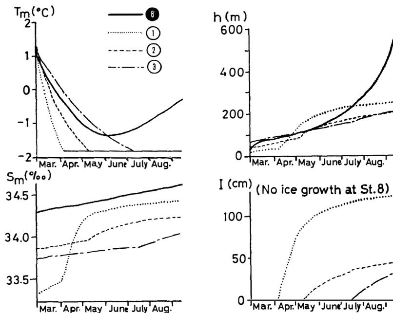
Fig. 3. Results of calculated variations of mixed layer temperature  $T_m$ , salinity  $S_m$ , thickness  $h$  and sea ice thickness  $I$  at Stns. 1, 2, 3 and 8 in 1974.
