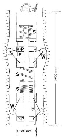
Fig. 1. Schematic illustration of the device. S: Compressive spring, W: Wheel, P: Rotational potentiometer, F: Rod for release.
