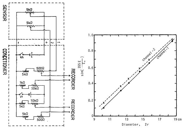
Fig. 3. Schematic diagram of the circuit Fig. 4. Result of laboratory tests. E: Output voltage,  $E_0$ : of measurement system. Input voltage (constant).
