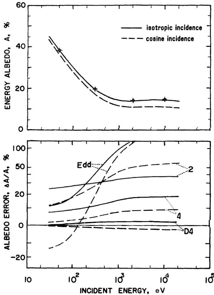
Fig. 3. Upper panel: Energy albedos, which include the contribution of secondary electrons and degraded electrons, shown as functions of the incident electron energy. Solid line (isotropic incidence) and dashed line (cosine incidence) are calculated from the double-Gauss 8-stream approximation. Symbol  $\oplus$  shows the results from the double-Gauss 4-stream approximation for the isotropic incidence.
