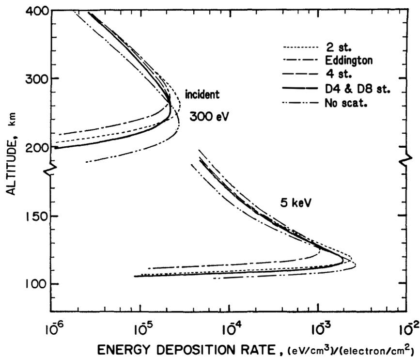
Fig. 2. Energy deposition profiles per unit number flux of incident electrons. The results calculated from several approximations are shown for the isotropic incidence of mono-energetic electrons at 300 eV and 5 keV.
