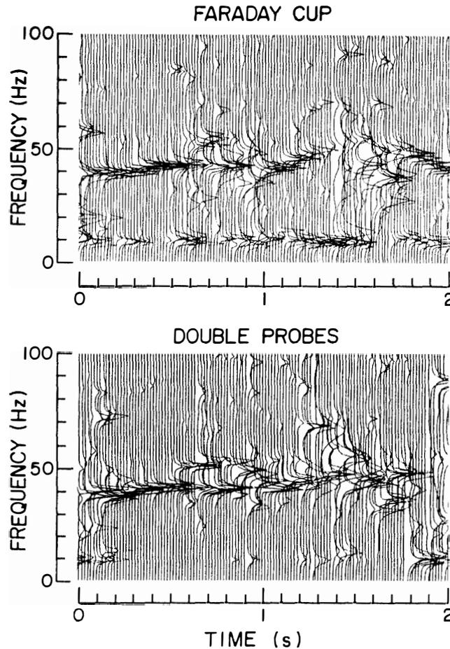
Fig. 1. Dynamic spectra of plasma density fluctuations measured by a Faraday cup (upper panel) and electric field fluctuations measured by a pair of double probes (lower panel) at the height of 210 km.
