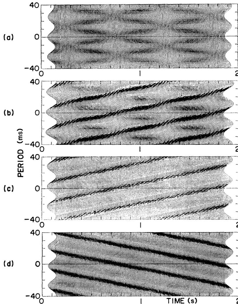
Fig. 4. Expected time variation of cross-correlation functions for (a) a plane, (b) a spinwise elliptically, (c) a spinwise circular, and (d) an anti-spinwise circular polarized waves where the frequency of the waves is 40 Hz, and the spin rate is 1 Hz.
