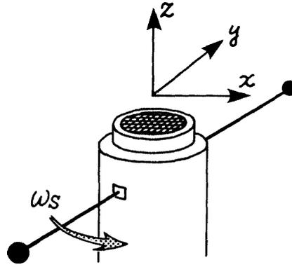
probes are deployed perpendicular to the rocket axis.
