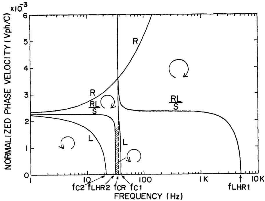
Fig. 5. Phase velocity-frequency diagram of electromagnetic wave modes calculated for the plasma of two ion species  $O^+$  and  $NO^+$ , where the phase velocity is normalized by the light velocity  $C$ .
