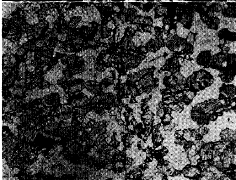
Fig. 6. Micrograph of Y-791195 eucrite showing gabbroic texture. Long axis is 5 mm, plane polarized light.
