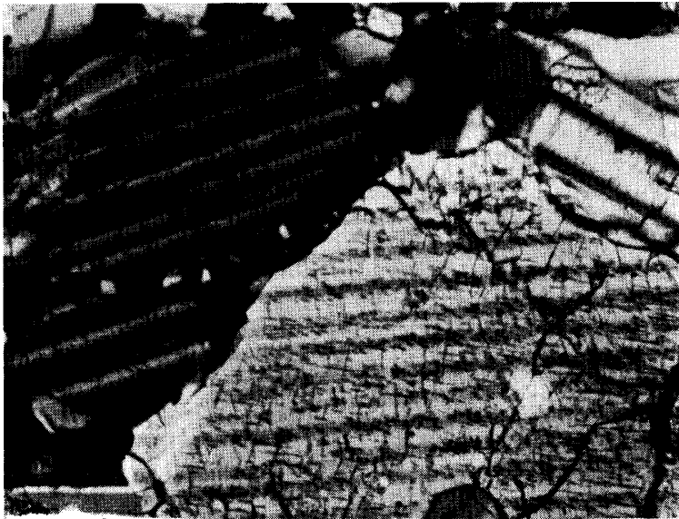
Fig. 7. Micrograph of Y-791195 simple lamellar exsolution and swarms of oriented inclusions. Long axis is 0.9 mm, crossed polarizers.
