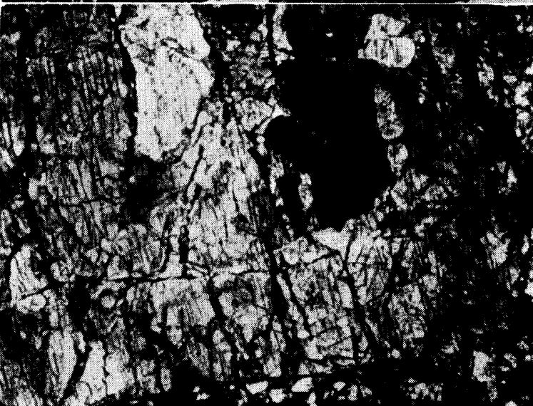
Fig. 9. Orthopyroxenite clast in Y-791186 containing three intergrown pyroxene grains. None are exsolved. Long dimension is 1.75 mm, crossed polarizers.
