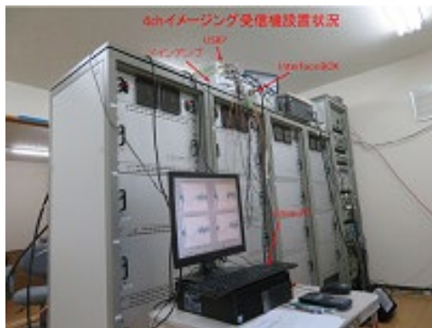
Figure 1. Photo of the 4-channel subset imaging receiver system installed at the SuperDARN Hokkaido East radar site.
