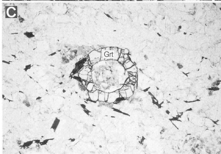
C : Photomicrograph of garnet-bearing granite (B86013105B). Loc.: Bergersenfjella. Open nicol. Width of photograph is 2.0 mm.
