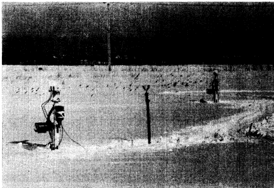
Fig. 2. Transmissometer installed above the snow surface with 30 m light path.
