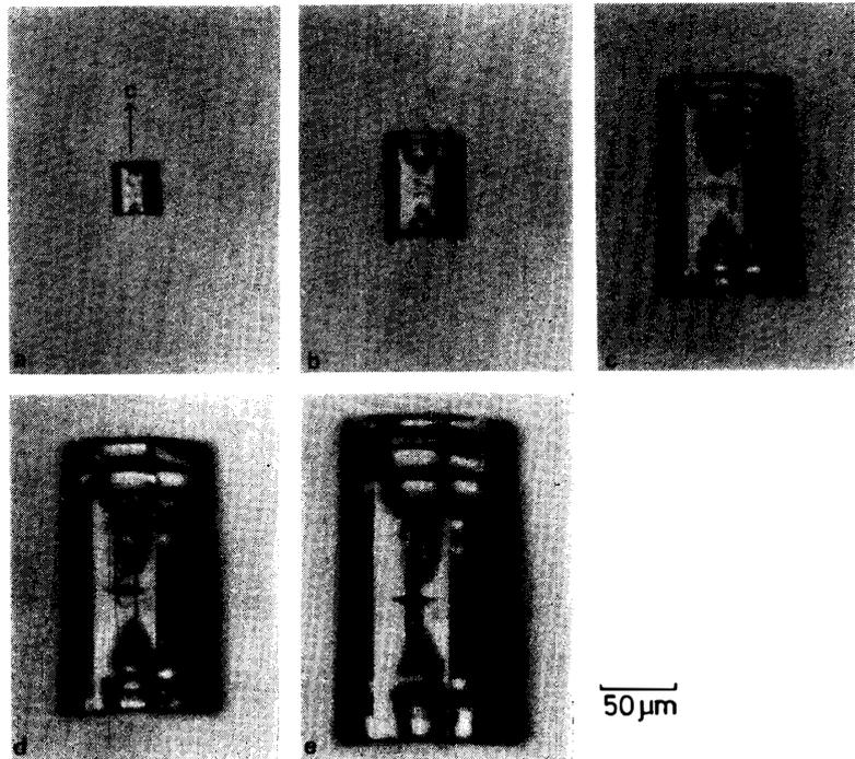
Fig. 3. Columnar ice crystal with skeletal structures grown in air at  $1.0 \times 10^5$  Pa at  $-30^\circ\text{C}$  and a supersaturation of 8.8%: (a) 1.8, (b) 14.3, (c) 60.5, (d) 92.0, (e) 142.9 min.
