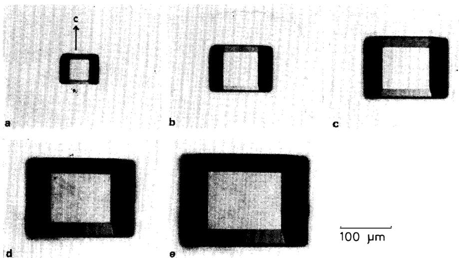
Fig. 2. Plate-like ice crystal grown in air at  $4.0 \times 10$  Pa at  $-30^\circ\text{C}$  and a supersaturation of 8.8%: (a) 0.4, (b) 0.8, (c) 1.2, (d) 1.7, (e) 2.3 min.
