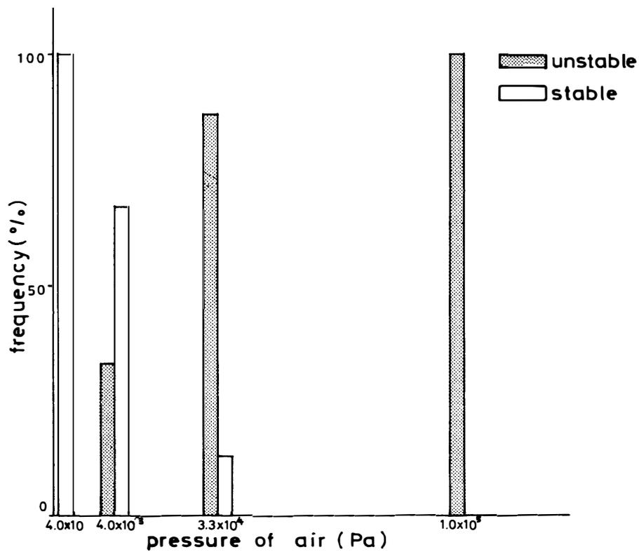
Fig. 4. Air pressure dependence of the instability of the (0001) face of  $80 \mu\text{m}$  columnar ice crystals grown at  $-30^\circ\text{C}$  and a supersaturation of 8.8%.
