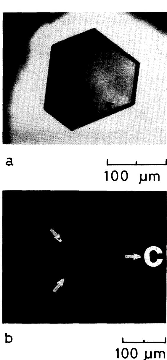
Fig. 7. Surface micromorphology of the (0001) and  $(10\bar{1}0)$  faces of ice crystals grown in air at  $4.0 \times 10^4$  Pa at  $-30^\circ\text{C}$ , (a) and (b) show the (0001) and  $(10\bar{1}0)$  faces, respectively; the arrow  $\uparrow$  is a spiral center.
