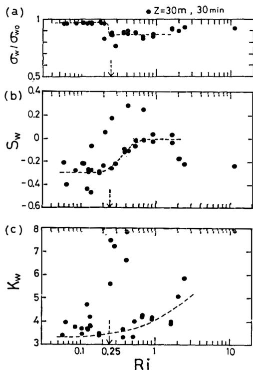
Fig. 6. (a) Relation between  $Ri$  and the ratio of filtered  $\sigma_w$  to  $\sigma_{w0}$  calculated from raw data of the  $w$  component at 30 m. (b) Filtered  $S_w$  as a function of  $Ri$ . (c) Filtered  $K_w$  as a function of  $Ri$ . Dashed lines in (a), (b) and (c) are eye-fits to the data of  $\sigma_w/\sigma_{w0}$ ,  $S_w$  and  $K_w$ , respectively.
