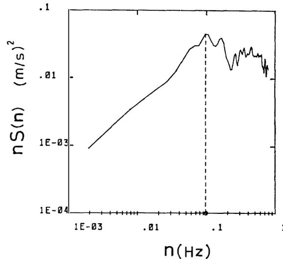
Fig. 5. Power spectra for the vertical wind velocity over the period 0300–0310, December 11, 1980 at 30 m at Nizuho Station. The peak frequency is indicated by the vertical dashed bar.
