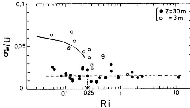
Fig. 3. Relationship between the vertical turbulent intensity ( $\sigma_w/U$ ) and gradient Richardson number  $Ri$  in the range  $0.05 < Ri < 12$ . The solid line shows KONDO *et al.*'s (1978) empirical relation at 3 m and the dashed line indicates  $\sigma_w/U = 0.015$ .
