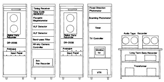
Fig. 3. A layout of the observation system at Husafell.
