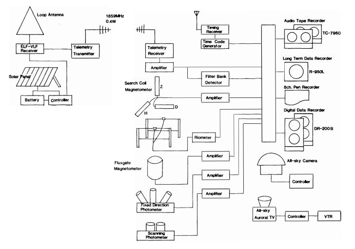
Fig. 2. Block diagram of the observation system at Husafell.
