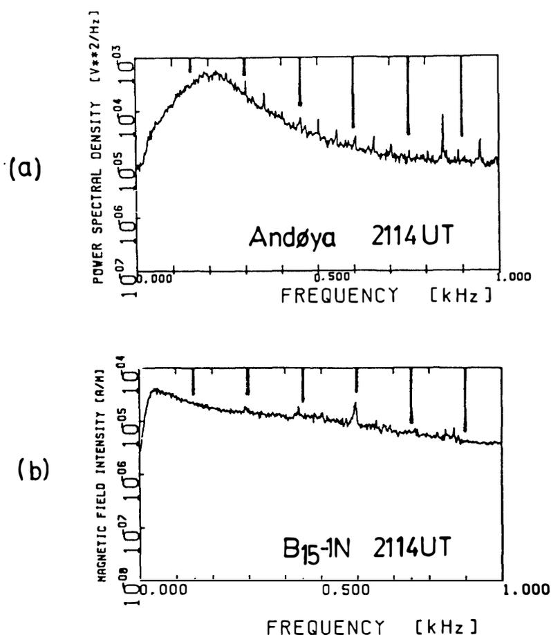
Fig. 6. Magnetic field spectra simultaneously obtained at 2114 UT on the ground station Andøya, Norway (a) and on balloon B<sub>15</sub>-1N flying over north Sweden (b). Many spectral peaks of harmonic frequency of 50 Hz can be seen up to 1 kHz in the spectrum (a). They are induced from local power lines. However, spectral peaks only at 300, 450 and 600 Hz are observed on the balloon as shown in (b).
