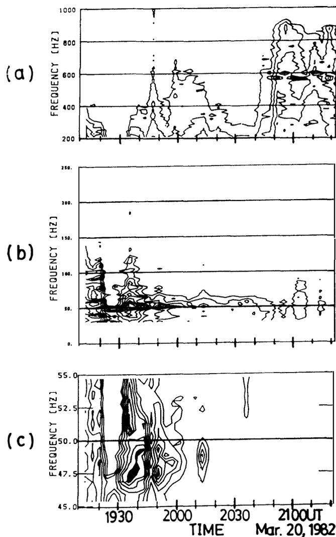
Fig. 5. Contour maps of the intensity of the magnetic field spectra observed on balloon  $B_{15-1N}$ . (a) Frequency range of 200 Hz to 1 kHz. (b) Frequency range of 0 to 250 Hz. The threshold level of indication is 10 dB greater than that of (a). (c) Magnification of the map (b) about 50 Hz which is the fundamental frequency of the power line radiation in northern Europe.
