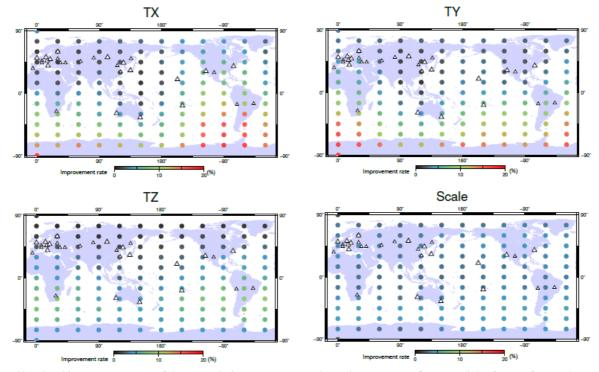
Fig. 2. Simulated improvement rate of three translation parameters and a scale parameter of a terrestrial reference frame when one laser-tracking station (one of the colored circles) is added to the existing laser-tracking network (white triangles; large ones are high productive stations) (Otsubo et al., 2016).
