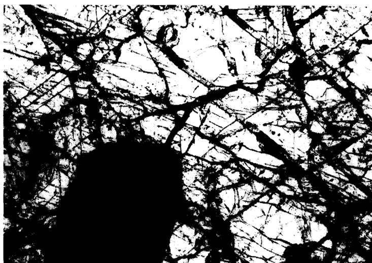
Fig. 1a. Photomicrograph of a large chromite crystal found in a crystalline clast of Shalka. Open. Width is 3.2 mm.
