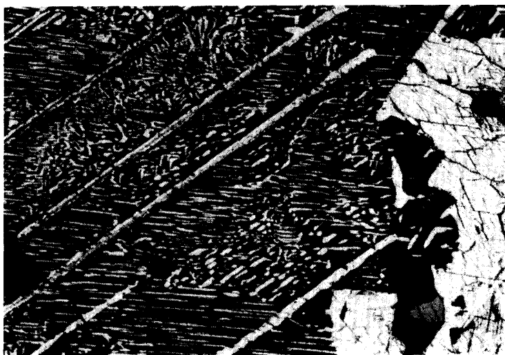
Fig. 3a. Photomicrograph of an inverted pigeonite from Serra de Magé. Width is 2.0 mm. Cross polarized light. Note orientations of augite blebs between the (001) augite lamellae.
