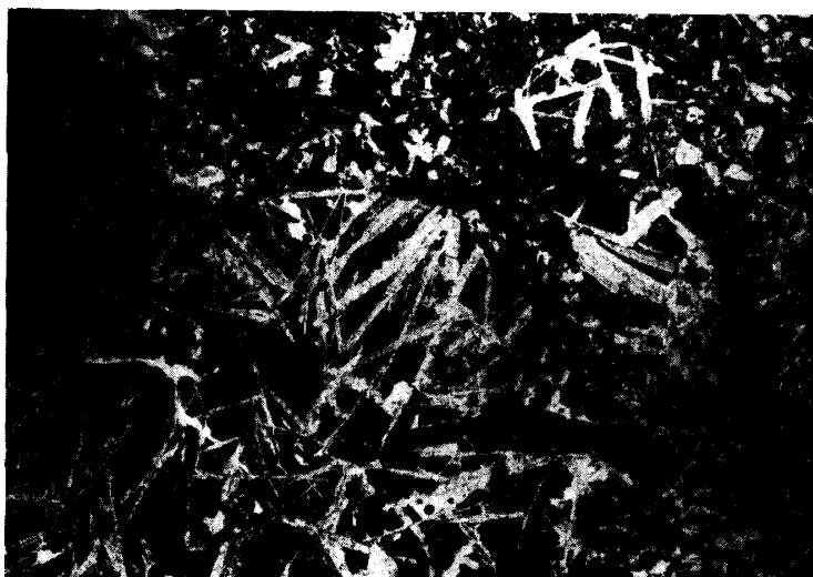
Fig. 14a. Photomicrograph of Nuevo Laredo. Fine-grained texture of a larger area than that in Fig. 14b. Width is 3.2 mm.
