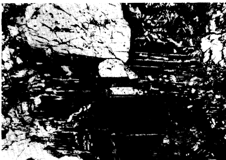
Fig. 2. Photomicrograph of Binda. Low-Ca inverted pigeonite with blebby inclusions of augite. Cross polarized light. Width is 3.2 mm.
