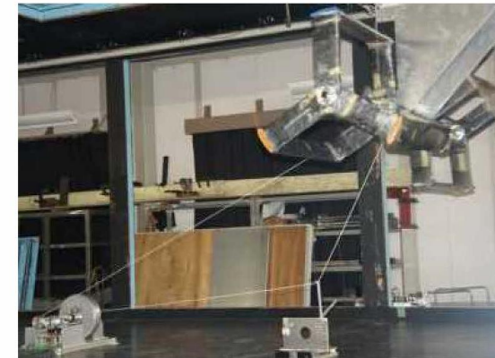
Wind tunnel test of phase 1.5 of HSWG at Kyusyu University (Test section 3.6 m \times 2.0 m) Windmill (diameter 0.6 m \times span 0.6 m \times 2) at the upper right is connected through tether to the generator on the lower left (13 September 2016).
