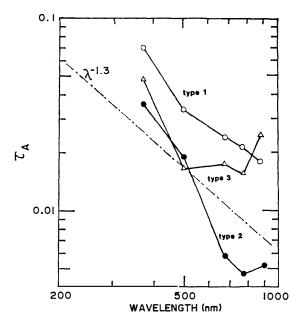
Fig. 3. Examples of aerosol extinction spectra in three types obtained at Syowa Station. A dotdash-line is evaluated by the power law spectrum.
