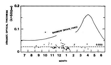
Fig. 2. A comparison of seasonal variation of aerosol optical thickness between Syowa Station and Barrow, Arctic (SHAW, 1982). Solid circles and crosses denote the data in the period from January to December 1980 and the data in January 1981 observed at Syowa Station, respectively.
