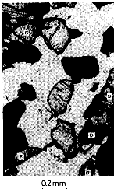
Fig. 3. Occurrence of garnet. Three garnets (high relief) are embedded in plagioclase aggregate. Plagioclase (white), hornblende (darker grain), Fe-Ti oxides (o), and salite (s) are seen. Attachment of salite with garnet as seen in this figure is a rare example throughout the slide.
