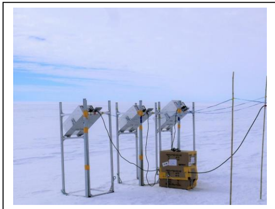
Figure 1. Microwave radiometers set at the S17 site, Antarctica.
