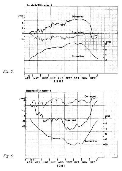
Figs. 5. and 6. Corrected ground tilt data of X- and Y-OUT.
