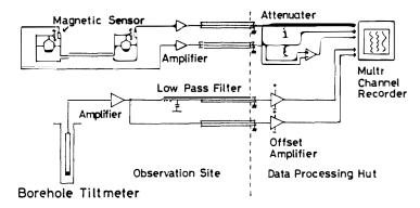
Fig. 3. Block diagram of the ground tilt observation. The borehole type and the water-tube tiltmeters are shown. The details of the water-tube tiltmeter are described by KAMINUMA and NAGAO (1983).
