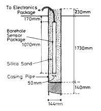
Fig. 2. A schematic view of the installation of the borehole type tiltmeter.
