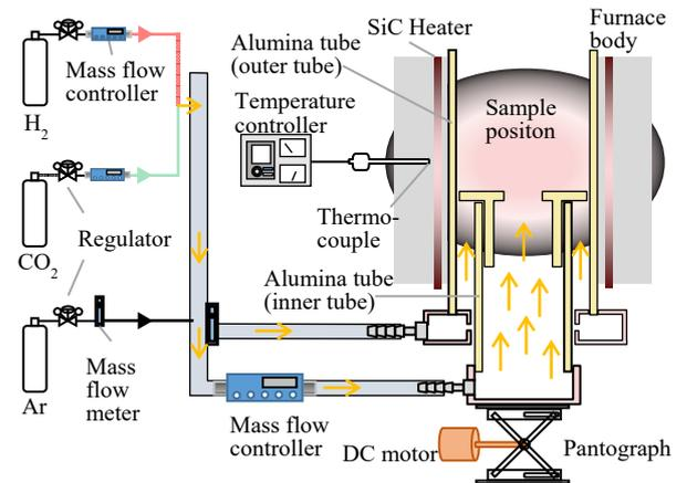
Fig.1. Schematic diagram of the present system.
