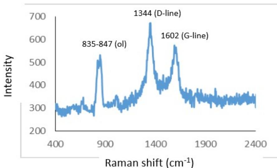
Figure 1. Raman spectral properties of the carbonaceous matrix with olivine.
