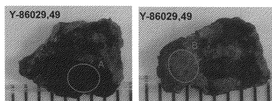
Fig. 1. Example images of measured spots on a Y-86029 chip sample viewed from two different sides, showing fresh dark Spot A and terrestrially-weathered light Spot B. The spot size is about 2 \times 3 mm, and the scale is 1 mm.
