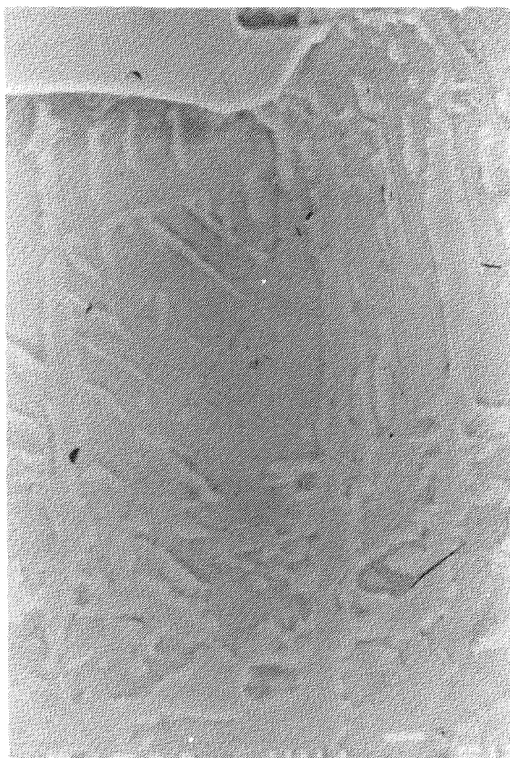
Fig.2 SEM photograph of shock-hatched kamacite
