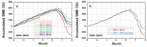
Figure 1. The NHM-SMAP-simulated (a) accumulated GrIS SMB during the 2010-2016 mass balance years, and (b) comparison of the model simulated accumulated SMB during the 2011-2012 mass balance year, where vertical water movement in snow and firn are calculated by the Richard equation (red solid line) or the bucket scheme (blue solid line) in the SMAP model.
