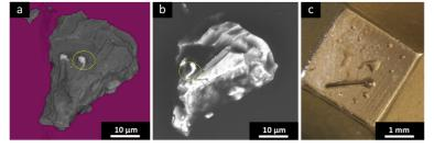
Fig. 1. Rehearsal using Kilabo particle. (a) 3D image of the sample obtained by SRCT. Some phases consisting of heavier elements show bright color. (b) BSE image of the same sample as in (a). (c) An image taken by optical microscope of the same sample. The sample was mounted on the potted butts with epoxy before C-coating.
