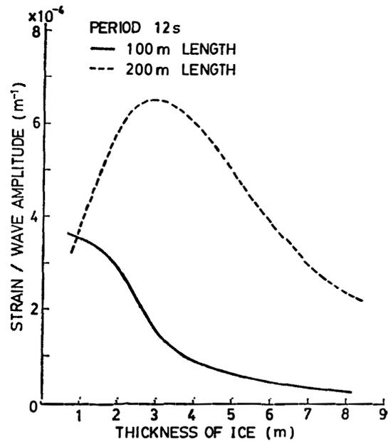
Fig. 3. Theoretical prediction of the strain/(wave amplitude) required to propagate a 10 mm crack for an ice plate of different thickness under action of swell of 12 s period.
