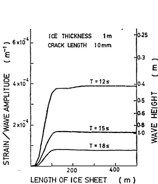
Fig. 2. Theoretical prediction of the strain/(wave amplitude), and wave height required to propagate a 10 mm crack for an ice plate 1 m thick as a function of length.
