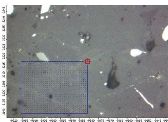
**Fig. 2.** The area of micro-Raman mapping. The blue rectangle area shows the grid network and contains 1044 measuring points.
