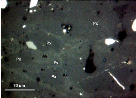
**Fig. 1.** OM-image (reflected light mode) of pyroxene (Px) and akimotoite (Ak) transformation area. The micro-Raman mapping was done in the left bottom corner.
