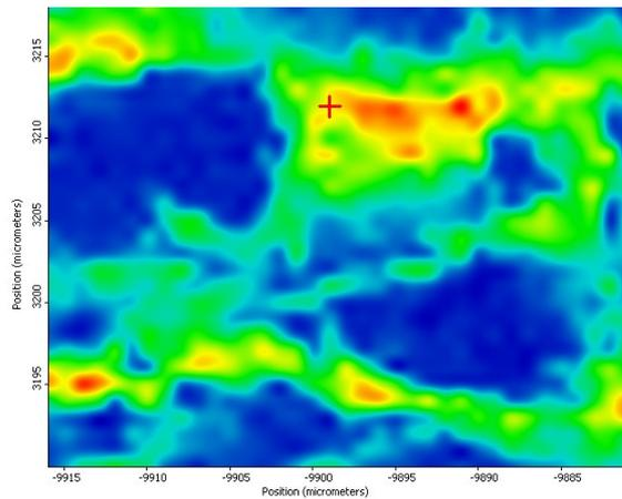
**Fig. 3.** Micro-Raman map which was created from 1044 spectra from blue rectangle area of Figure 2. The color variation from blue to red shows gradually growing intensity for  $800\text{ cm}^{-1}$  major peak of akimotoite.
