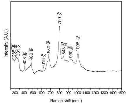
**Fig. 4.** Micro-Raman spectrum of akimotoite lamella from NWA 5011 chondritic meteorite.
