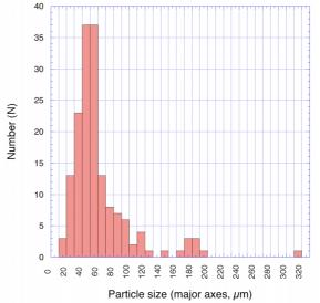
Fig. 2. A size distribution of Hayabusa ferromagnesian silicate particles. It shows a peak in the size range from 50 and 60  $\mu$ m. A depletion of particles sized less than 50  $\mu$ m might result from technical difficulty in manipulation of such small particles.
