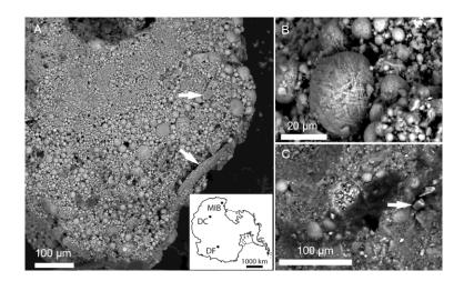
Fig. 1: Back scattered electron image of the aggregates of meteoritic ablation spheres from Miller Butte, Victoria Land Transantarctic Mountains studied in this work (obvious bedrock crystals embedded in the aggregates are arrowed). A) Sample #20c.25. B) Close-up of sample #20c.25 showing spherules with dendritic textures. C) Sample #20c.351. Inset: sketch map of Antarctica showing the location of Miller Butte (MIB), and Dome C and Dome Fuji where similar spheres were found in ice cores [2, 3].
