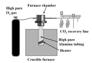
Figure 1. The extremely low level <sup>14</sup>C extraction system for HED meteorites at Rissho University
