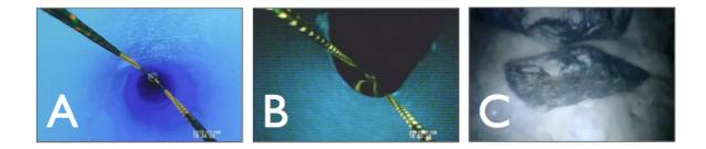
Fig.1 Borehole video images. A: Interior features of the borehole; B: Boundary between fresh water and seawater; C: Glacial erosional boulders within fine marine sediments on the sea flor.
