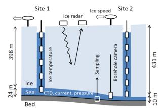
Figure 2. Schematic diagram showing the longitudinal cross section of the studied region of Langhovde Glacier. Filed measurements performed on, within, and beneath the glaciers are depicted.
