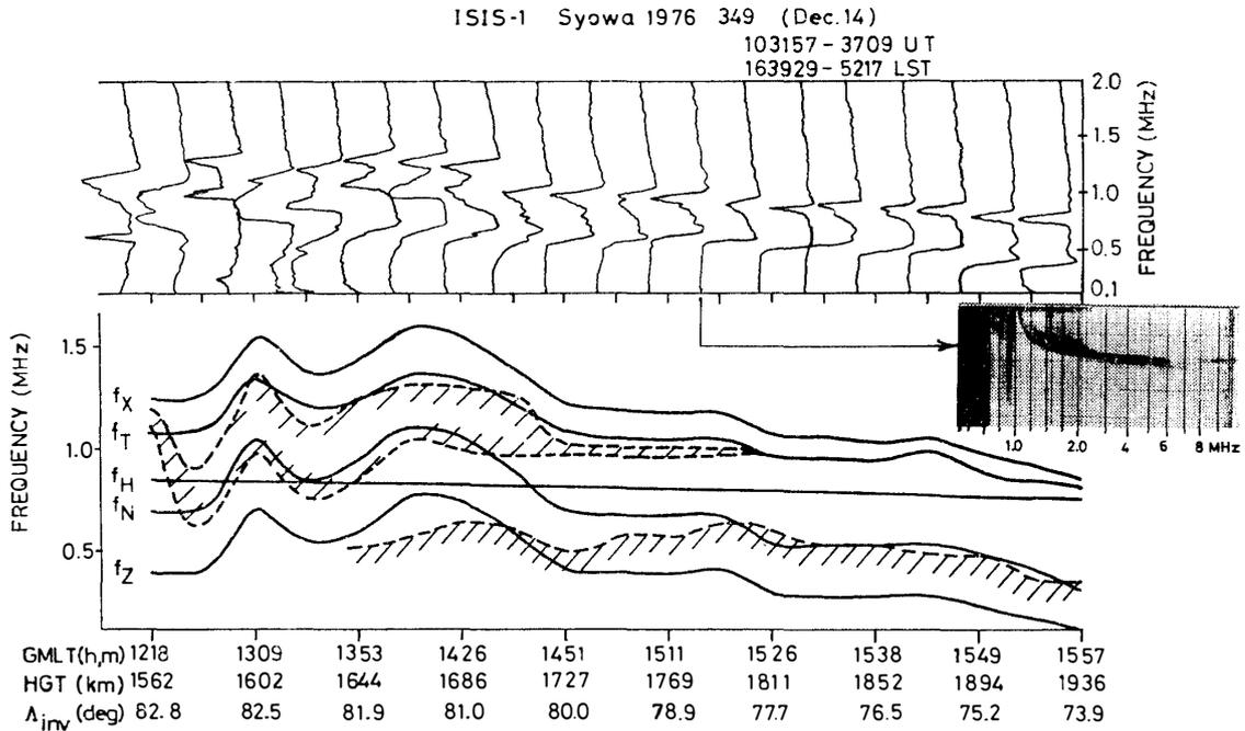
Fig. 4. A series of ISIS-1 AGC sweeps and the relationship between the frequency range of noise exceeding a certain threshold level and local characteristic frequencies  $f_N$ ,  $f_H$ ,  $f_T$ ,  $f_X$  and  $f_Z$  scaled on ionograms. Two kinds of noise can be seen in these spectra.
