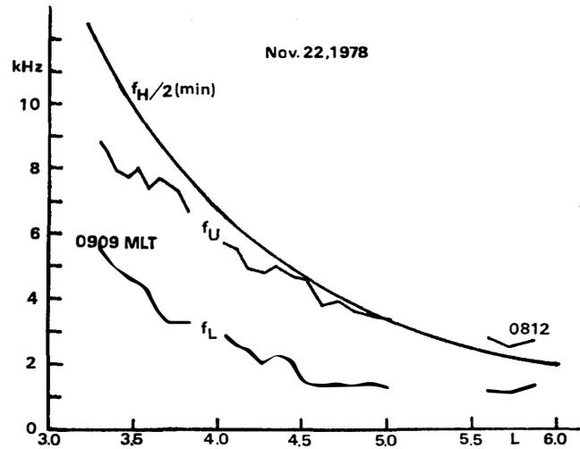
Fig. 2. Latitudinal (or  $L$ ) variation of the dayside chorus band frequency observed in the local evening on November 22, 1978 by ISIS-2 and latitudinal (or  $L$ ) variation of one half the equatorial electron gyrofrequency.
