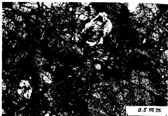
Fig. 8. A group of shear fissure and its rhombic knot phenomenon in the Jilin meteorite.
