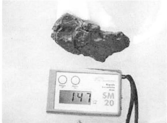
**Fig. 2.** One of ordinary chondrites found in Moulton Escarpment by KOREAMET. The bottom is magnetic susceptibility (MS) meter showing that the meteorite is relatively high in MS and probably H-group.
