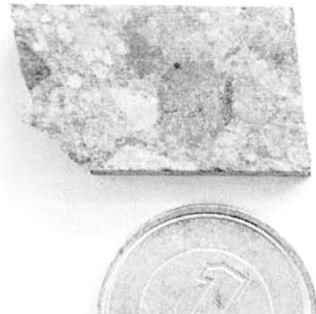
Figure 3 A rock sample of NWA1794 (LL5) after nano-second pulse laser irradiation. The laser pulse power was 15 mJ. The size of darkened irradiated area is 6 mm.
