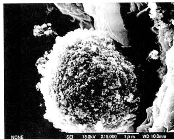
Fig4. Electron micrograph (BEI) of Ni-Fe spherules (31%Ni and 29%Fe). Nickel is mixed with Fe. The samples are the same in Fig.2.
