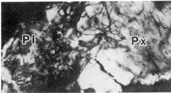
Fig. 2. Photomicrograph of the heated Zagami “maskelynite” for 72 hours (crossed polarizers). The original maskelynite converts to polycrystalline plagioclase (left). The field of view is about 550\mu\text{m} . Pl: plagioclase. Px: pyroxene.
