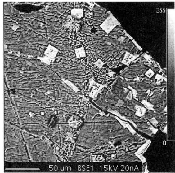
Figure 2. BSE image of a halite grain (grey) containing cubes of sylvite (white), from the Monahans 1998 H5 chondrite.
