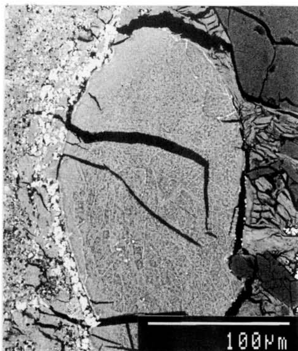
Fig.6: Typical texture of the fine-grained, Cr-rich inclusions (compare Fig.5; BSE-image)
