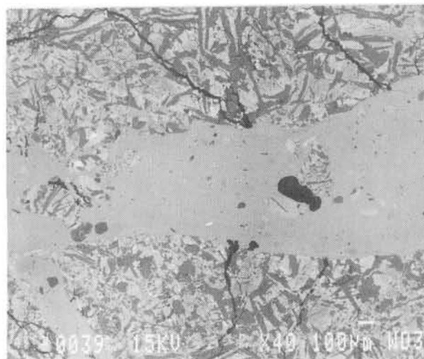
Fig.2 BEI of the shock melt vein of swirly glass in Y-82202. Black crystals : plagioclase. White crystals : pyroxene. Gray area in the middle : shock melt vein.
