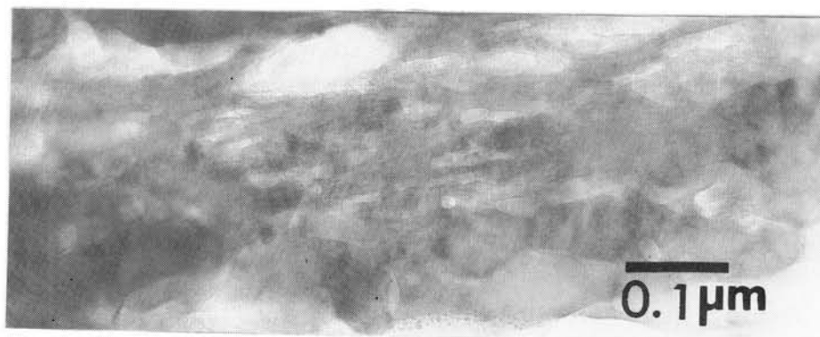
Fig. 1 Thermally affected saponite grains in B-7904 matrix.
