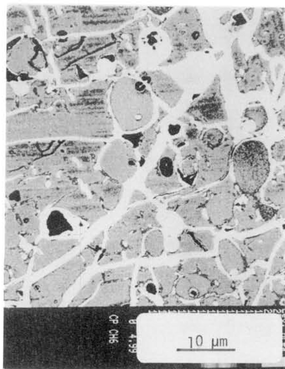
Fig.2 BEI of low-Ca pyroxene phenocryst in a chondrule (Y-790112). "Banding" or "lines" are shown in pyroxene.
