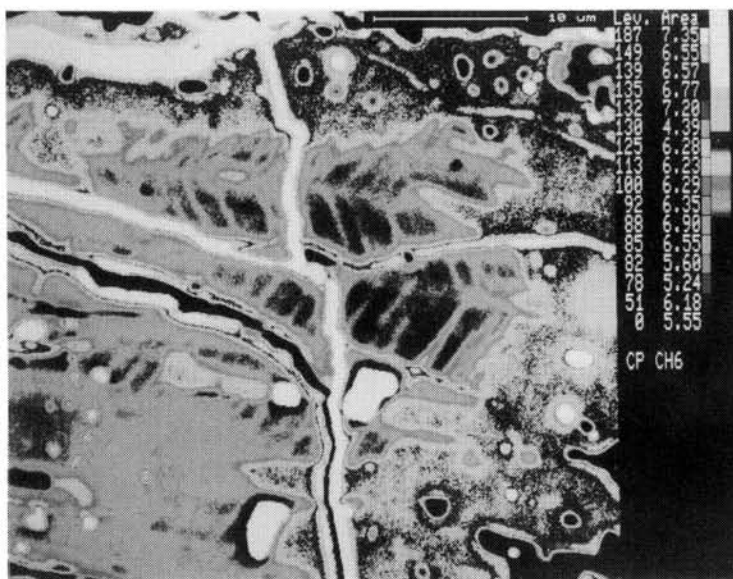
Fig.1 BEI of "pigeonite" shows exsolution lamellae. Lamellae are herringboned by twinning of "pigeonite". (Y-74115, H5)
