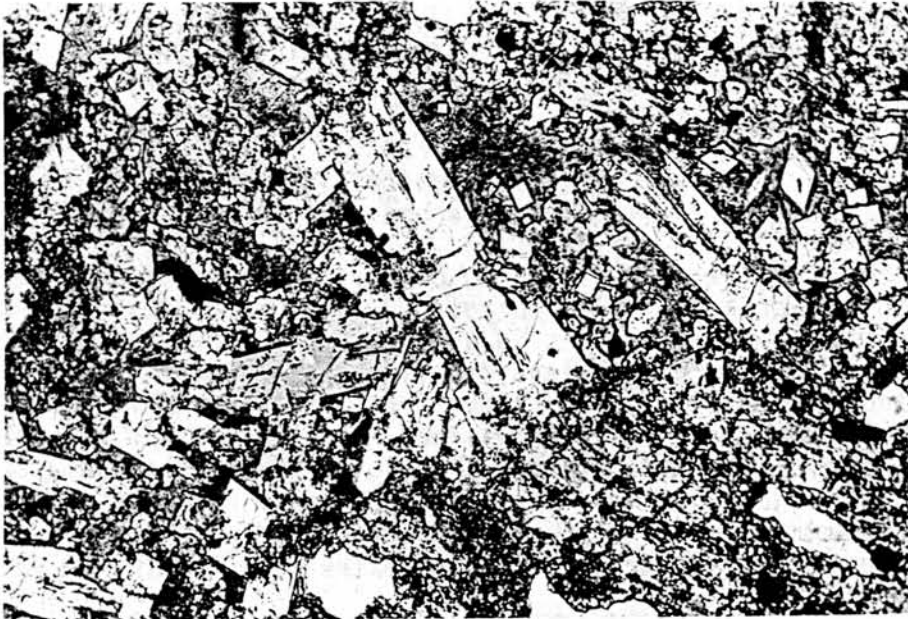
Fig. 1 Photomicrograph of Y-790964. Euhedral pyroxene crystals are embedded in an extremely comminuted mineral fragments and the brown-colored glass. These pyroxenes show Ca-enrichment at the rim. Width: 0.8mm
