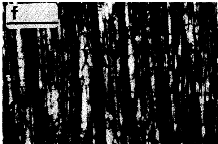
Fig. 5f. Same as Fig. 5e. Close-up. Polysynthetic twin is easily recognized.
