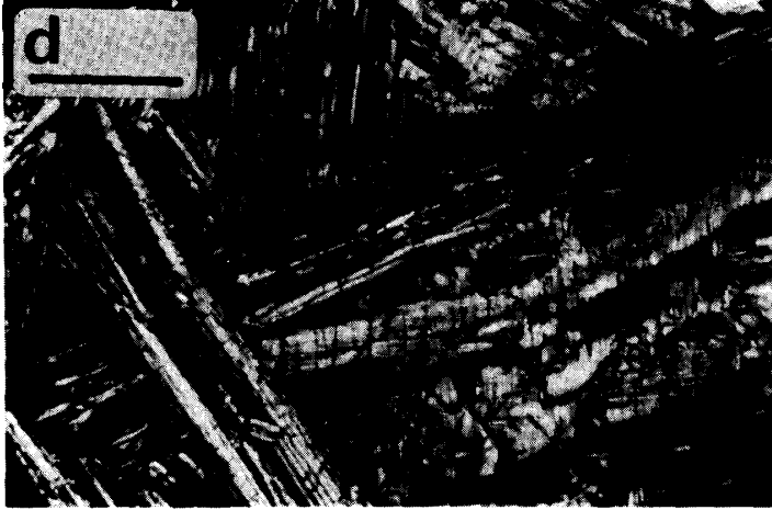
Fig. 5d. Run 574, cooled at 125°C/hr. Barred-radial olivine texture.
