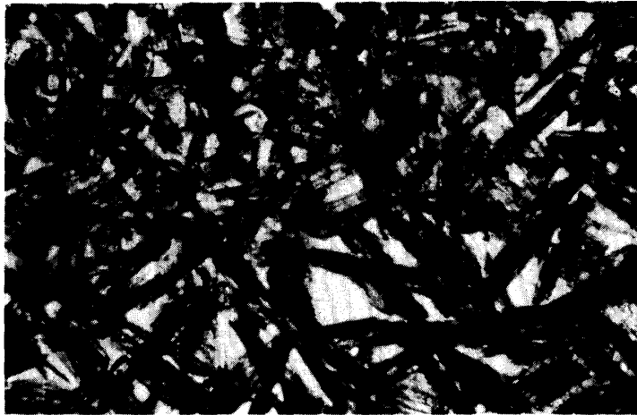
Fig. 3g. Run 535, cooled from 1445°C. Aggregates of acicular olivine crystals.
