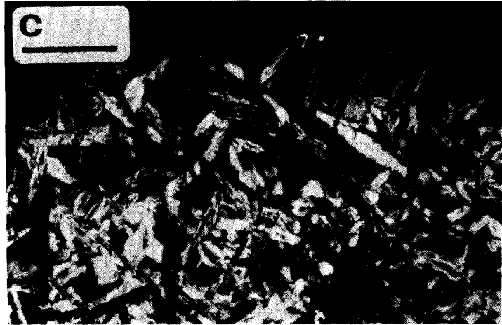
Fig. 2c. Run 505, quenched from 1568°C. Relict olivine rimmed by quench crystals is present.
