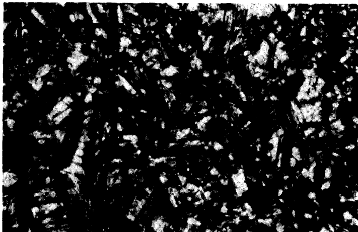
Fig. 3h. Run 533, cooled from 1440°C. Aggregates of acicular olivine crystals.
