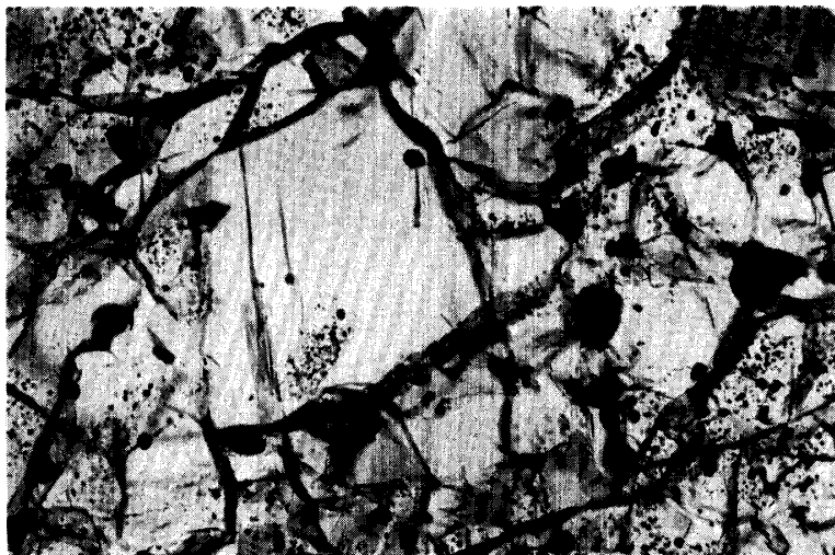
Fig. 10b. Very large clear orthopyroxene in a narrow coarse-grained vein in Yamato-74013. Width is 0.80 mm.
