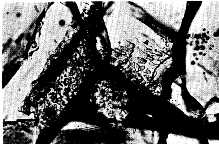
Fig. 6b. Enlarged view of the graphic textures exhibited by plagioclase and silica mineral assemblages at the middle left edge in Fig. 6a. Width is 0.20 mm.
