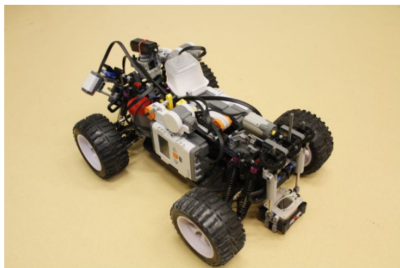
Fig. 3. The Husar-5 rover with the Carbonate experiment when coil of the magnetic experiment is in lowered position.
